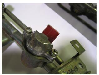
Tighten by hand the two hold down screws evenly, alternating screws until hand tight. Torque screws to manufacturers specification.
